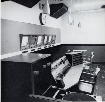
FIG. 24. View of a control booth from clients' booth. Audio position includes RCA BC-2B Audio Console and RCA BCM-11A Mixer Console, and two RCA BQ-70B Transcription Turntables.
