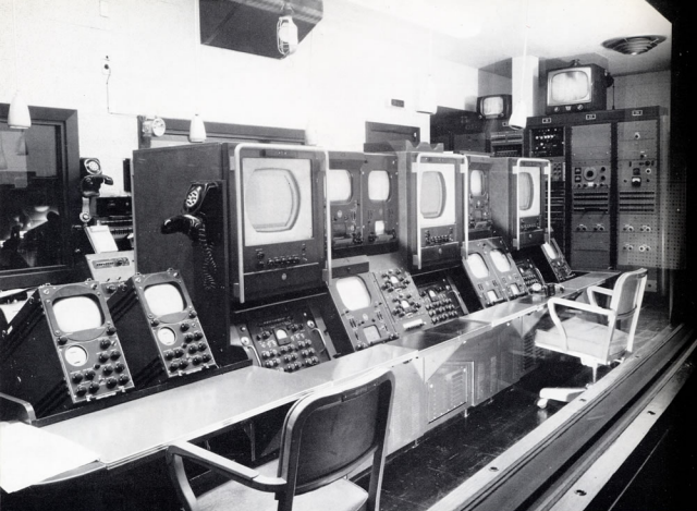
FIG. 18. WBTV's video control console as seen through the window from the a-m control room (see floor plan, Fig. 6). Camera control for four monochrome studio cameras, one color studio camera, two 3-V color film cameras and two color Chromascan units are incorporated in this console. Monitors are provided for both monochrome and color operation. Location of the various units in this console is shown in Fig. 19. Video operators at this position make all necessary camera adjustments. Camera switching is done by the director in the studio control booth.
